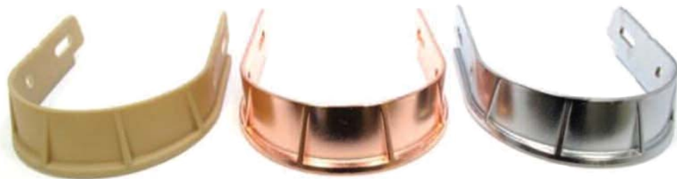
Fig. 4 — Nanometal/polymer hybrid heel cups showing the bare, copper-metallized, and Nanovate-coated stages.
