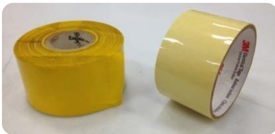
Traditional electroplaters tape (L) and custom electrical tape (R)
