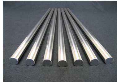
Figure 14: nCoP plated steel bars prior to machining and assembly.
