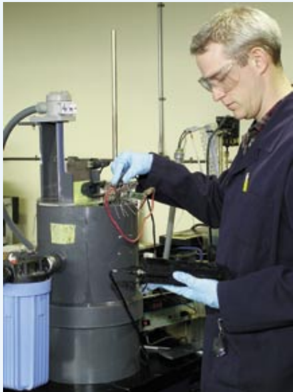
Nanomaterials are enhancing surface finishing technologies in many applications. Integran's Iain Brooks is shown here operating the plating cell for production of Nanoplate® materials.
